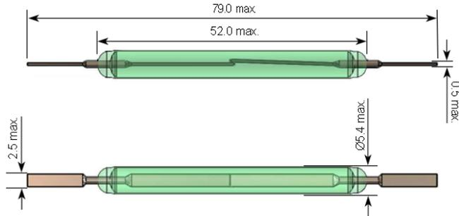
tolerances according to DIN ISO 2768 m
