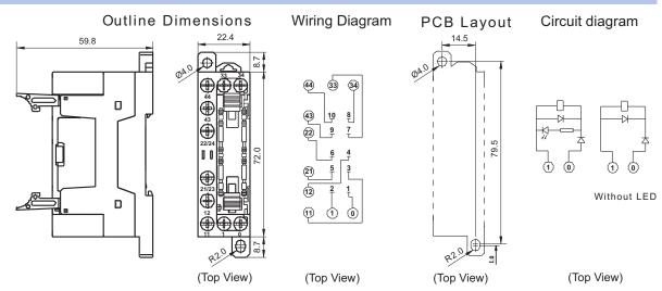
Notes: Main outline dimension(L, W, H)  $\geqslant$ 50mm, tolerance should be  $\pm$ 1mm; outline dimension >20mm and <50mm, tolerance should be  $\pm$ 0.5mm; outline dimension  $\leqslant$ 20mm, tolerance should be  $\pm$ 0.3mm.
