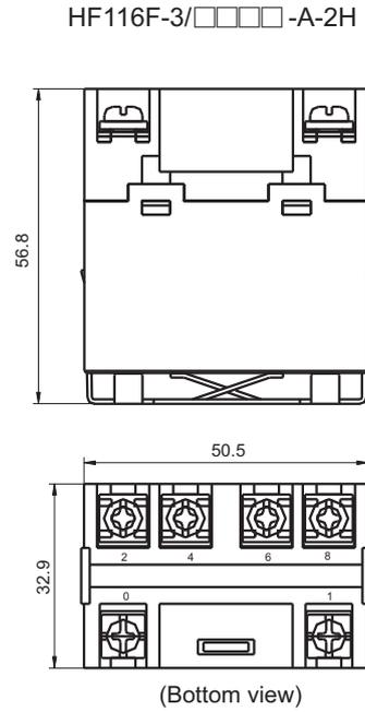
Remark: In case of no tolerance shown in outline dimension: outline dimension  $\leq 1\text{mm}$ , tolerance should be  $\pm 0.2\text{mm}$ ; outline dimension  $> 1\text{mm}$  and  $\leq 5\text{mm}$ , tolerance should be  $\pm 0.3\text{mm}$ ; outline dimension  $> 5\text{mm}$ , tolerance should be  $\pm 0.4\text{mm}$ .
