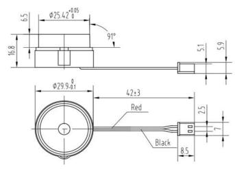
Connector Housing: A2503HOO-2P Connector crimp: A2503TOP-2
